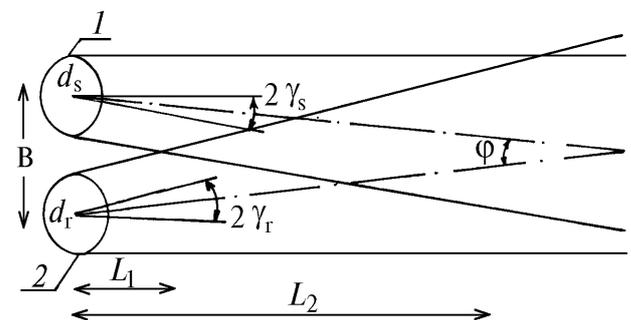
FIG. 1. Geometrical scheme of lidar visibility meter. Source aperture (1) and receiver aperture (2).
