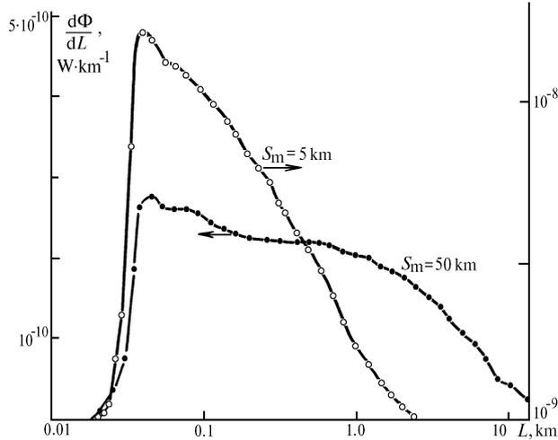
FIG. 2. Differential fluxes of backscattered radiation. Opto-geometrical parameters of lidar visibility meter:  $P_0 = 4.5 \cdot 10^{-2}$  W,  $2\gamma_s = 5'$ ,  $d_s = 0.005$  m;  $2\gamma_r = 1^\circ$ ;  $d_r = 0.1$  m,  $B = 0.2$  m;  $\varphi = 0^\circ$ .
