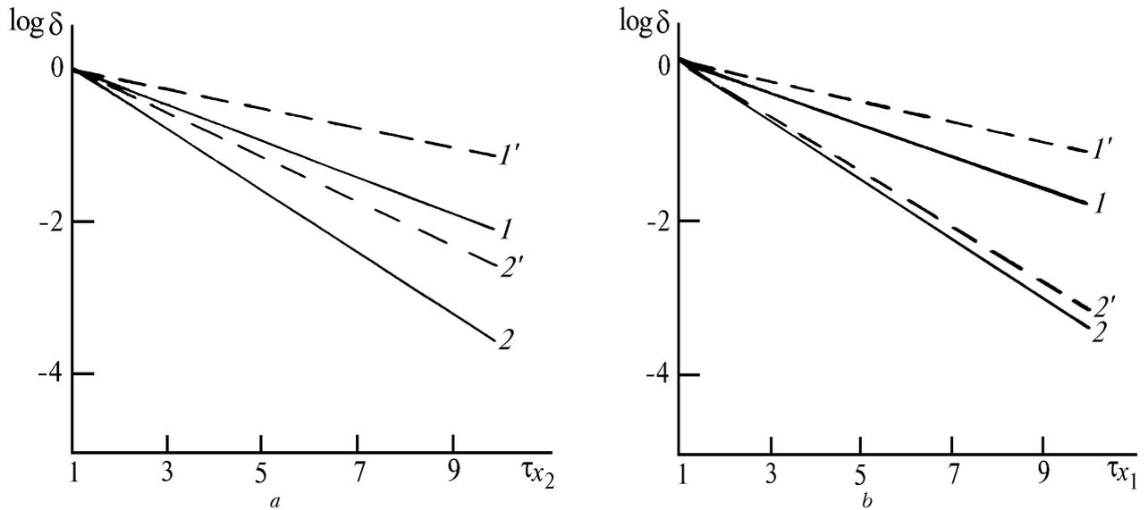
FIG. 1. Signal-to-noise ratio vs. the optical depth of the medium at  $\tau_{y,z} = 5$ : a)  $a_2=1, a_1=a_3=12$  (1 and 1');  $a_2=12, a_1=a_3=1$  (2 and 2');  $\Lambda=1$  (1 and 2) and 0.8 (1' and 2');  $\tau_{x_1}=\tau_{x_3}=1$ ; b)  $a_2=12, a_1=a_3=1$  (1 and 1');  $a_2=1, a_1=a_3=12$  (2 and 2');  $\Lambda=1$  (1 and 2) and 0.8 (1' and 2');  $\tau_{x_2}=\tau_{x_3}=1$ .
