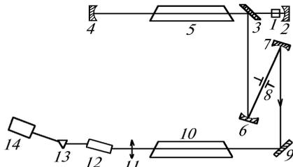
FIG. 1. Diagram of the setup for conversion of CVL emission in nonlinear crystal.
