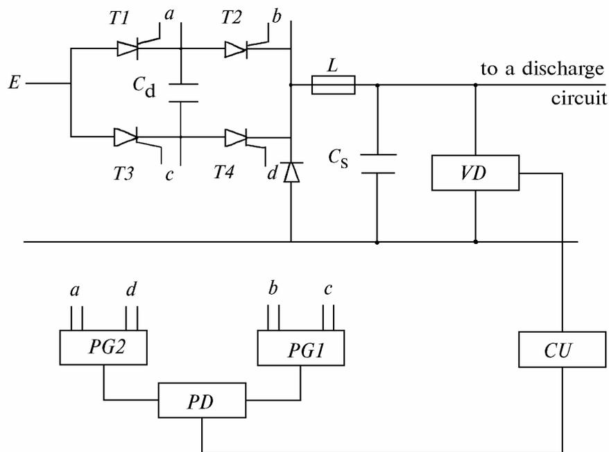
FIG. 1. Block diagram of a charger with fixed voltage across the dosage capacitor.
