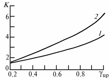
FIG. 4. Dependence  $K = f(\gamma_{up})$  for the two–range (1) and three–range (2) systems at  $\alpha = 0.1$ .
