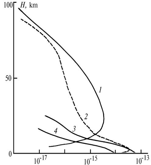
FIG. 4. Altitude dependence of the weighting function at  $dT/dz$  for several frequencies:  $\nu = 2360.8$  (1),  $2379.27$  (2),  $2392.35$  (3), and  $2424 \text{ cm}^{-1}$  (4).
