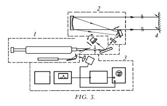
The lidar employs a cw  $CO_2$ -laser (1) discretely tunable over vibrational-rotational transitions, a transmitting and receiving optical system (2), and electronic equipment for recording signals (3). The laser frequency modulation within a chosen vibrational-rotational transition contour is done by changing the cavity length by means of oscillations of a mirror fixed on a piezocorrector.
