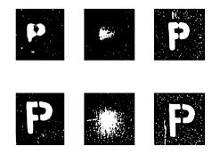
FIG. 4. Examples of quality of optical images recorded through a scattering layer: upper raw is for milky medium and lower is for mat glass.
