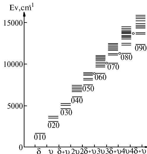
FIG. 5. Diagram of the vibrational states of the  $H_2O$  molecule. Open circles denote highly excited local resonances.
