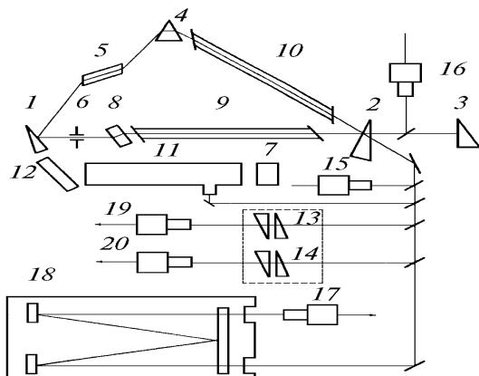
FIG. 1. Block-diagram of a high-resolution laser spectrophotometer with Nd:glass ring-cavity laser. 1, 2, and 3 are the cavity mirrors; 4 is the prism; 5 is the active laser media; 6 is the diaphragm; 7 is the optical multichannel analyzer; 8 is the plane-parallel plate; 9 and 10 are the cells; 11 and 12 are the polychromator; 13 and 14 are the Fabry-Perot interferometer; 15, 16, 17, 19, and 20 are the photodetectors; and, 18 is the multipass cells.
