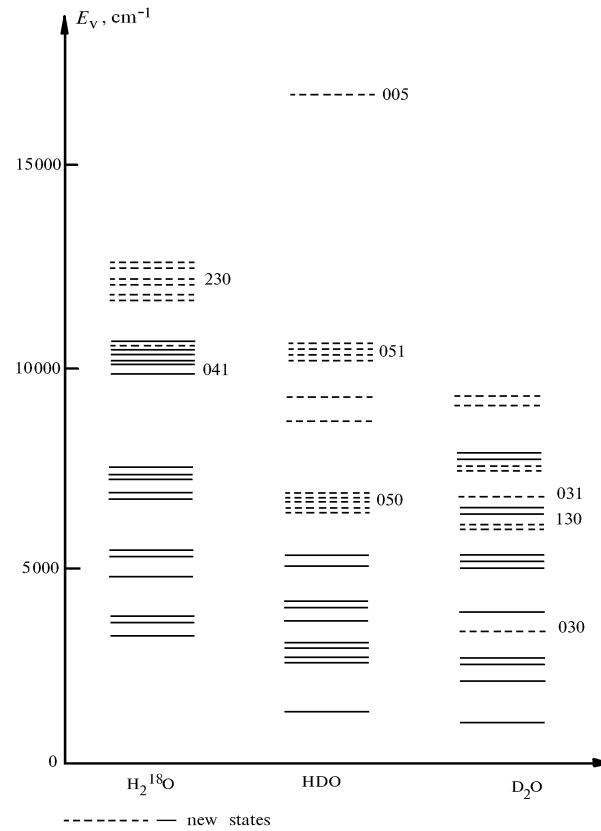
FIG. 6. Vibrational states of water molecule isotopomers (dashed lines denote the bands investigated at IAO).
