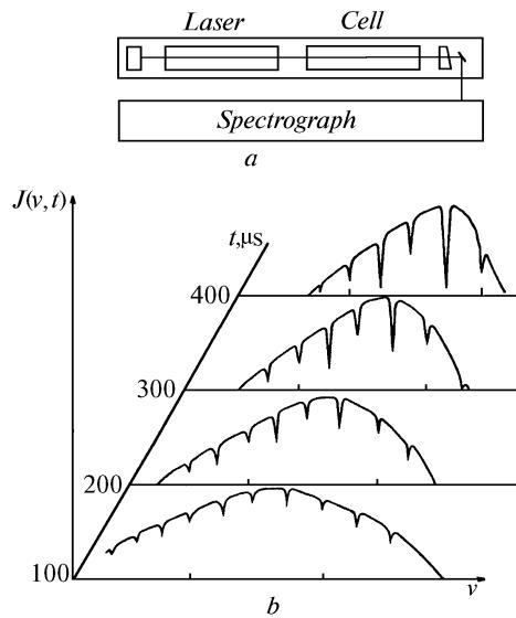
FIG. 2. Block-diagram of an ICL spectrometer (a). Emission spectrum of a broad-band laser with the selective intracavity losses at different time moments (b).
