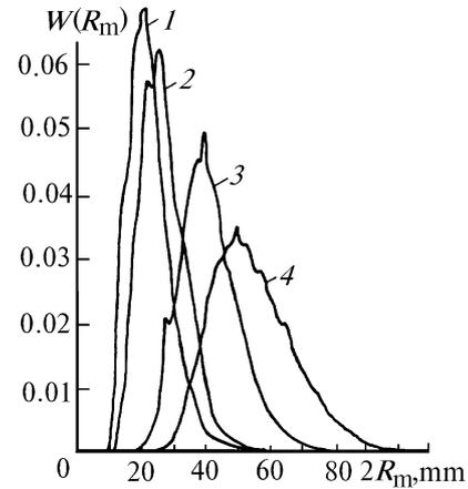
FIG. 2 Histograms of probability density of fluctuations of the instantaneous beam radius  $R_m$  for  $C_n^2 = 3.6 \cdot 10^{-15}$  (1),  $5.1 \cdot 10^{-15}$  (2),  $1.1 \cdot 10^{-14}$  (3), and  $2.2 \cdot 10^{-14} \text{ m}^{-2/3}$  (4).
