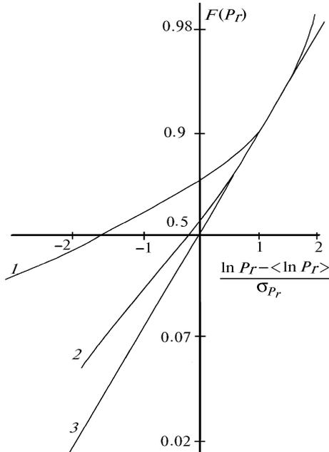
FIG. 4. Probability distribution of the received power fluctuations for wandering (1) and nonwandering (2) beams and the lognormal distribution (3).
