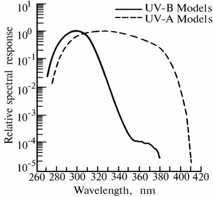
FIG. 1. Relative spectral response of the Model UVB-1 pyranometer.
