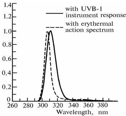
FIG. 2. Convolution of the solar irradiance spectrum with erythemal action spectrum and the relative response of the Model UVB-1 pyranometer.
