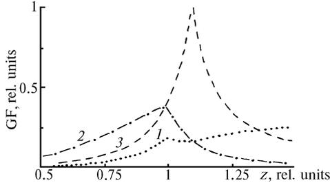
FIG. 4. Formation of the geometrical function for a bistatic two-lens transceiving objective: the resultant GF (1), beam overlapping coefficient (2), and image transfer ratio (3).
