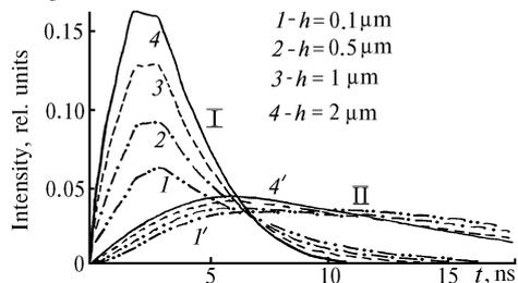
FIG. 2. Calculated signals recorded with the fluorometer for oil products with short ( $\tau = 1$  ns) (I) and a relatively long decay time ( $\tau = 10$  ns) (II) for the films of different thickness.
