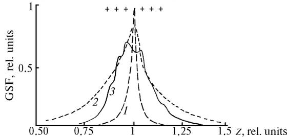
FIG. 5. Examples of geometrical functions: for sounding depth of 5 m and for a single-lens receiving objective (1), for sounding depth of 25 m and a single-lens receiving objective (2), for a 6-lens objective and sounding depth of 5 m (3).
