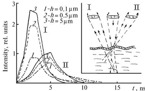
FIG. 6. Calculated signals for a bistatic sounding scheme: signals in the informative channel (I) and signals in the channel recording the background fluorescence (II).
