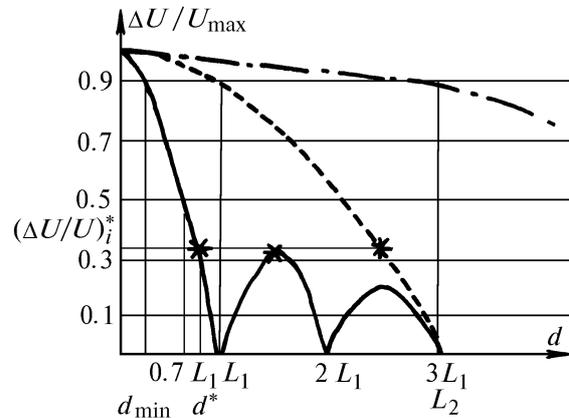
FIG. 1. Dependence of the function  $(\Delta U / U_{\max})$  on the particle diameter for different periods of the interference pattern (the method of polychromatic equidistant bands).
