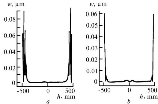
FIG. 2. The residual wave aberration of the Schmidt system for the correctors shown in Fig. 1: a) profile 1 and b) profile 2.
