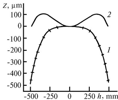
FIG. 1. Correction planoid profile of the Schmidt system: 1) profile of the corrector located in the center of a spherical mirror; 2) profile of the corrector displaced at a distance of 7.5 mm.
