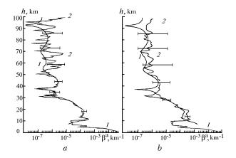
FIG. 2. Initial (1) and reconstructed (2) scattering coefficients  $\beta^{\alpha}(h)$ : Tikhonov method (a) and Volz–Goody method (b).
