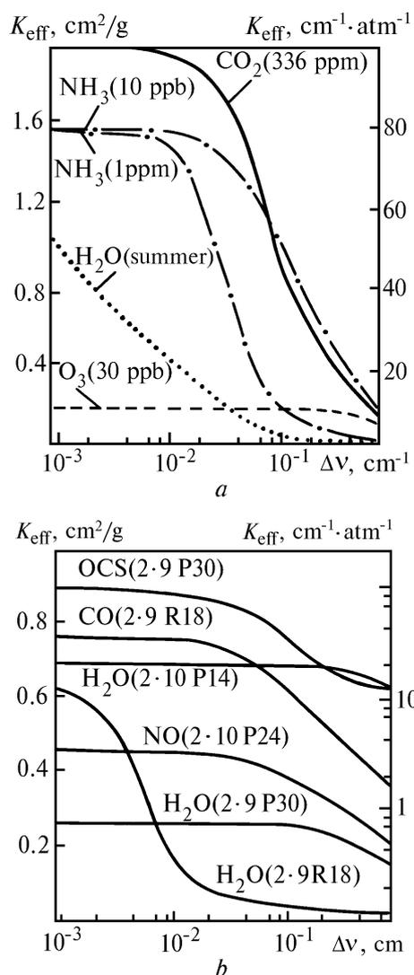
FIG. 1. Dependence of the effective absorption coefficients of the indicated gases on the CO<sub>2</sub>-laser line width in the spectral regions of the first (a) and second (b) harmonic of the CO<sub>2</sub> laser.
