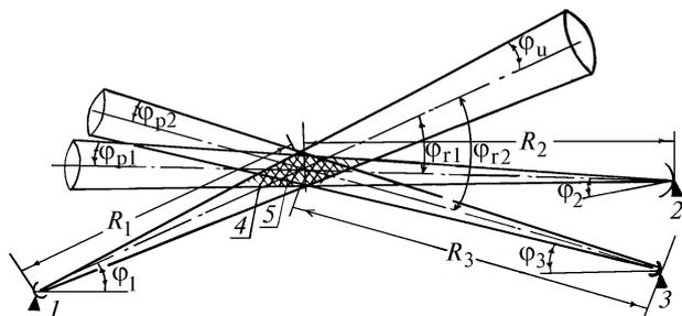
FIG. 3. Geometry of the experiment. Here 1 is the sound source, 2 and 3 are the receivers, and 4 and 5 are the scattering volumes.
