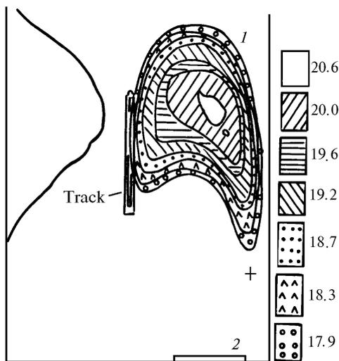
FIG. 5. Thermogram of the transient regime with the particle track shown to the left: discharge 1 and electrode 2.
