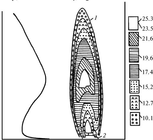
FIG. 1. Thermogram of the stationary discharge 1 formed by the pointed electrode 2.
