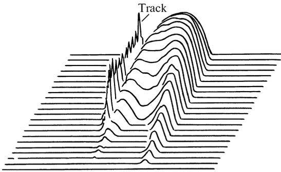
FIG. 4. Three-dimensional double-humped thermogram in the transient regime. To the left of the figure, the particle tracks are shown.
