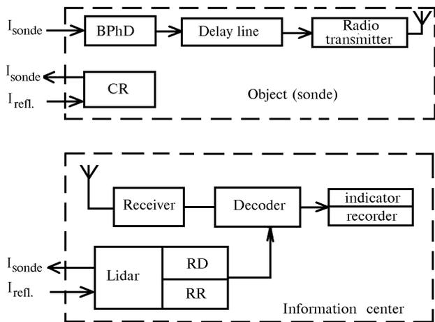
FIG. 1. Block diagram of the device for identification of an object number.
