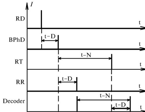
FIG. 2. Time diagrams of functioning of the device for identification of an object number.
