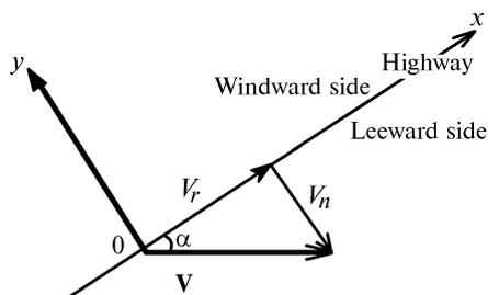
FIG. 1. Geometrical relationships between the wind and road directions:  $V$  is the wind vector,  $V_n$  and  $V_r$  are the projections of the wind vector to the road direction ( $x$ ) and to the direction normal to it ( $y$ -axis);  $\alpha$  is the angle between the road and the wind vector directions.
