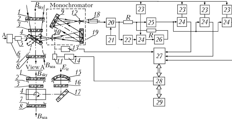
FIG. 1. Functional optoelectronic diagram of the measurer of the sea spectral radiance.
