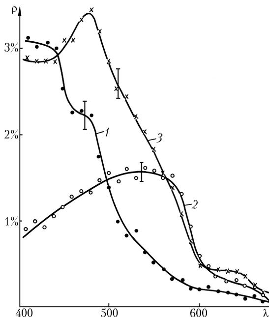
FIG. 2. Spectral dependences of the sea radiance coefficient measured with the three-channel spectrophotometer from aboard the research ship Akademik Kurchatov (53rd voyage, 1994) in the Aegean Sea (1), the Sea of Marmara (2), and the Black Sea (3).
