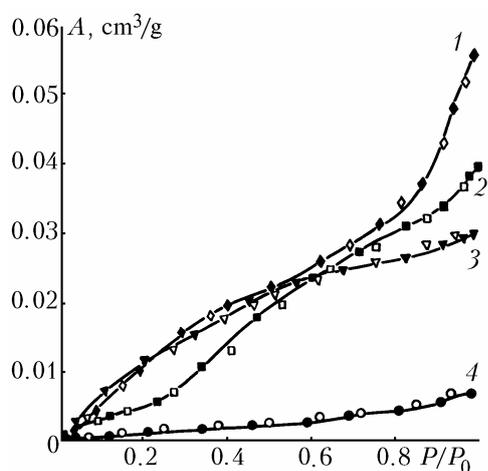
FIG. 3. Experimental isotherms of water vapor adsorption at a specimen temperature of 25°C for soot produced by burning of pine-tree wood (1), oil (2), natural gas (3), and pure carbon generated by evaporation of carbon rods in the arc discharge plasma (4); the closed symbols correspond to the adsorption branch, while the open ones are for the desorption branch.
