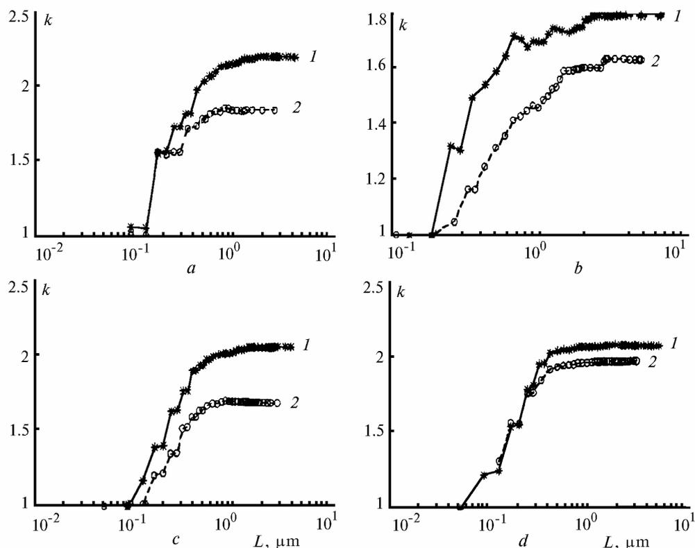
FIG. 2. The cluster size dependence of the shape anisotropy coefficients for the soot produced by burning pine-tree wood (a), natural gas (b), oil (c), and pure carbon generated by evaporation of carbon rods in arc discharge plasma (d): before (1) and after (2) the exposure to water vapor.
