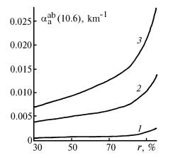
FIG. 1. Dependence of the submicron aerosol absorption coefficient in the 10.6  $\mu$ m range on the relative air humidity for three versions of  $\alpha_a^{ab}(10.6)$  calculations ( $m_d = 1.143$ ,  $\varkappa_d = 0.07$  (1);  $m_d = 1.5$ ,  $\varkappa_d = 0.7$  (2);  $m_d = 1.5$ ,  $\varkappa_d = 1.5$  (3)).
