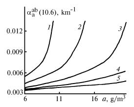
FIG. 2. Dependence of the submicron aerosol absorption coefficient in the 10.6  $\mu$ m range on the absolute air humidity for  $m_d = 1.5$ ,  $\varkappa_d = 0.7$  and five values of air temperature t = 12, 18, 24, 30, 36°C (curves 1, 2, 3, 4, 5, respectively).
