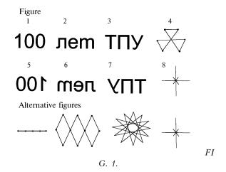
Note: Figures 5, 6, 7, 8 were generated with an output mirror (for writing on clouds). Instead of the figures 1, 2, 3, 4 or 5, 6, 7, 8, alternative figures can be generated provided that MC chips are changed.
