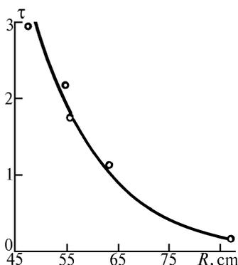
FIG. 3. Transition part radius  $R$  as a function of  $\tau$ .
