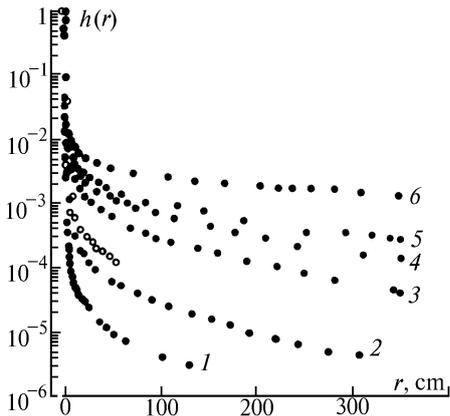
FIG. 2. PSF of the vision system as a function of  $\tau$  for wood combustion smokes: 1)  $\tau = 0$ ; 2) 0.16; 3) 1.12; 4) 1.74; 5) 2.16; 6) 2.94;  $\circ$  is for winter haze.
