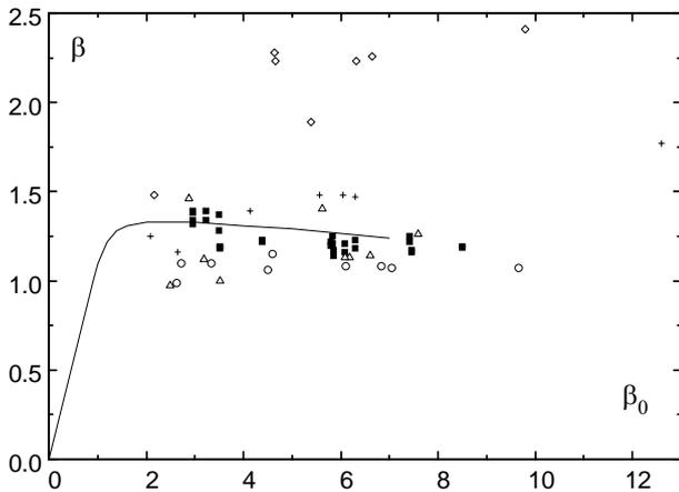
FIG. 1. Scintillation index of the intensity fluctuations  $\beta$  as a function of the parameter  $\beta_0$ : 1 corner-cube ( $\diamond$ ), 4 corner-cubes ( $+$ ), 16 corner-cubes ( $\Delta$ ), 26 corner-cubes ( $\square$ ), and flat mirror ( $\blacksquare$ ).
