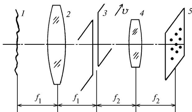
FIG. 1. Block diagram of the multichannel slit analyzer of a wave front of optical radiation.
