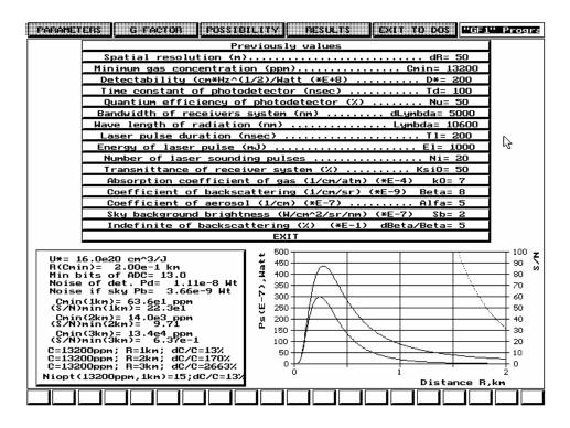
FIG. 4. Energy parameters and returns of IR DIAL.<sup>5</sup>
