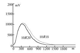
FIG. 2. Lidar returns for  $CO_2$  laser lines 10R20(ON)and 10R18(OFF) obtained along horizontal path on October 20, 1989, 10:00 LT at air temperature of  $18^{\circ}C$ and relative humidity of 72%. The data are taken from Ref. 5.
