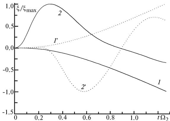
FIG. 2. Relative displacement of the surface of water droplets with  $r_0 = 0.03$  (1, 1') and  $3 \mu m$  (2, 2') as functions of time. Two directions are considered: along, at  $\theta = 0^\circ$ , (solid curve) and across,  $\theta = 90^\circ$ , the beam (dashed line) with the intensity  $I_0 = 10^8 W/cm^2$ , and pulse duration  $t_p = 10^{-7}$  sec.
