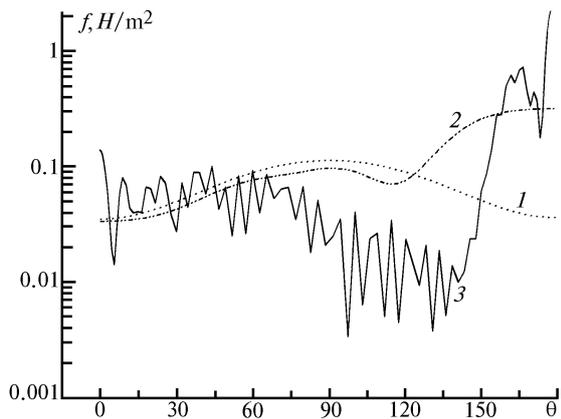
FIG. 1. The density of the normal component of the resultant pondermotive force on the surface of water droplets with the radius  $r_0 = 0.03$  (1),  $0.3$  (2), and  $3 \mu m$  (3) as a function of polar angle  $\theta$ . Z-axis is directed along the direction at  $\theta = 0-180^\circ$ . The incident radiation intensity was taken to be  $I_0 = 10^4 W/cm^2$ .
