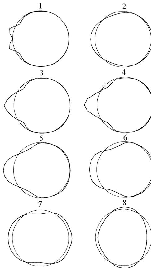
FIG. 4. The shape of the water droplet surface (main cross section) with  $r_0 = 25 \mu m$  at different time moments since the beginning of the action of radiation ( $I_0 = 10^9 W/cm^2$ ;  $t_p = 10^{-7}$  sec, direction of incidence from left to right):  $t = 50$  (1),  $80$  nsec (2),  $0.2$  (3),  $0.5$  (4),  $5$  (5),  $15$  (6),  $30$  (7) and  $40 \mu s$  (8).
