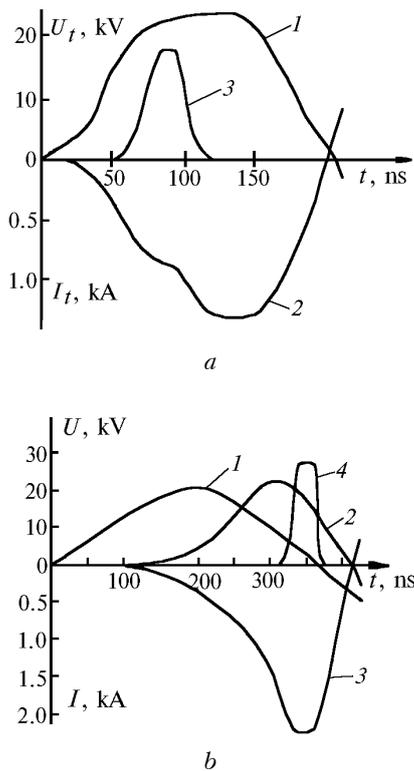
FIG. 2. Oscillograms of pumping pulses and laser output for two types of power sources: a) oscillogram of pulses of voltage at the tube,  $U_t$ , (curve 1) and current (2) in GDT laser with magnetothyristor source and laser radiation pulse (3),  $P_{Ne} = 110$  Torr; b) oscillograms of pulses of voltage at  $C_2$  (curve 1),  $C_3$  and GDT (2), current in GDT (3) and laser radiation pulse (4) for a laser with thyatron source  $P_{Ne} = 75$  Torr.
