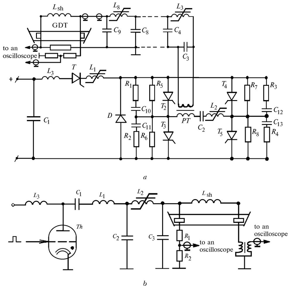
FIG. 1. Circuitry of two power supply sources for a copper-vapor laser: a) simplified circuitry of magnetohyristor power supply source of a laser GDT,  $C_3 - C_9 = 3.3$  nF; b) circuitry of a thyatron power supply source of a laser GDT,  $C_1 = 6.0$  nF,  $C_2 = 4.0$  nF,  $C_3 = 3.08$  nF.
