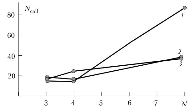
FIG. 7. Speed of control in a linear medium as a function of the number of degrees of freedom of an adaptive corrector. Numbers of curves are the same as in Fig. 6.
