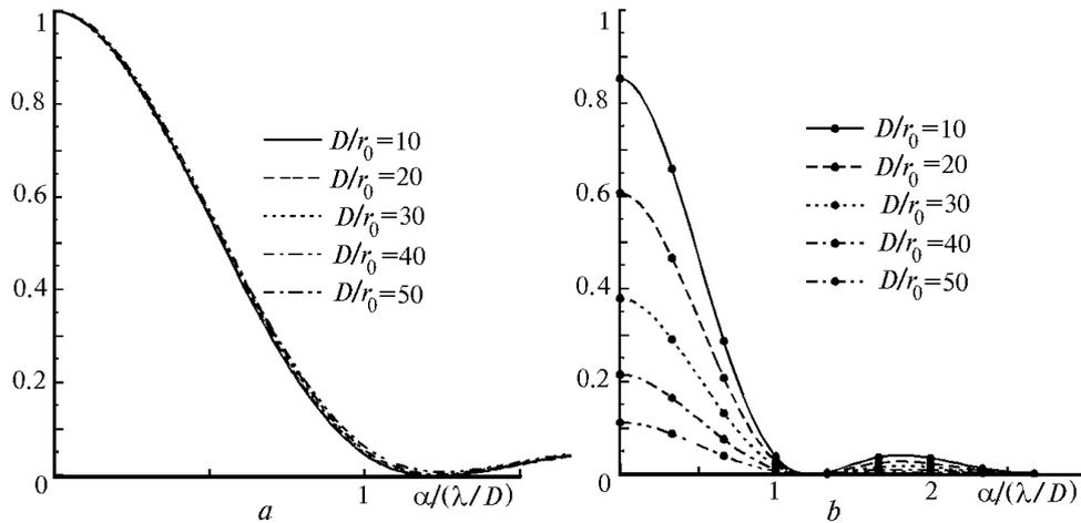
FIG. 4. AST-10 PSF, when the segmented adaptive mirror with 84 elements of hexagonal form is used. Every segment is controlled by the position and slopes. a – PSF is normalized by its axial value. b – PSF is normalized by the diffraction maximum.
