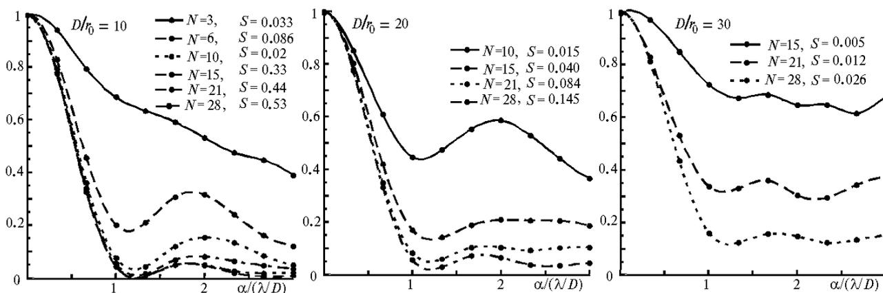
FIG. 2. AST-10 PSFs, when a modal corrector is used. Parameter  $N$  corresponds to the number of Zernike polynomials. PSF is normalized to the axial value.  $S$  is the Strehl ratio.
