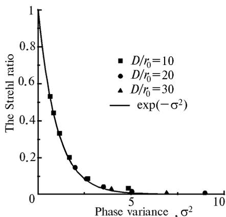
FIG. 3. The Strehl ratio as a function of the variance of phase residual distortions.
