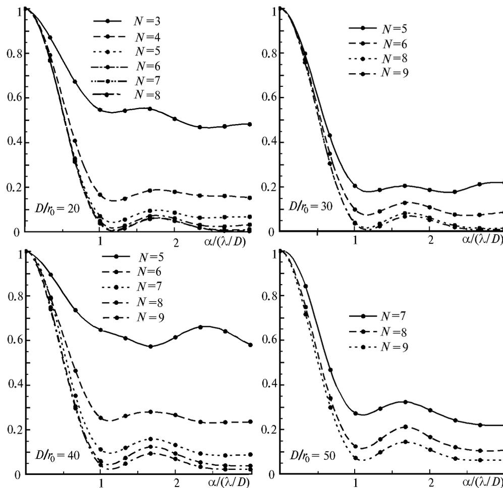
FIG. 5. AST-10 PSF, when a flexible adaptive mirror with the Gaussian reference function is used. Parameter  $N$  corresponds to a number of the control points at the aperture diameter. PSF is normalized by its axial value.
