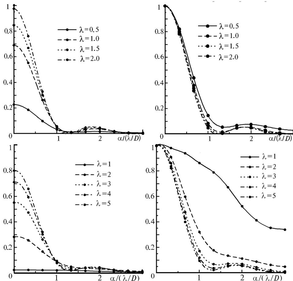
FIG. 7. PSFs of the AST-10 at different wavelengths for the adaptation using a laser reference star. Upper plots are for the sodium LRS ( $H = 100$  km), the lower plots are for the Rayleigh LRS ( $H = 10$  km). At the left plots the PSF is normalized to the diffraction maximum, at the right plots the PSF is normalized to its axial value. The wavelength  $\lambda$  is given in  $\mu\text{m}$ .
