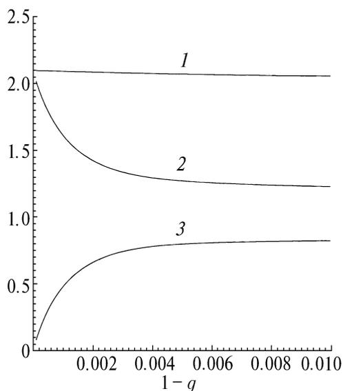
FIG. 1 Dependence of the extinction, scattering, and absorption factors of the particle with  $r = 10 \mu\text{m}$ ,  $n_1 = 1.33$ ,  $\kappa_1 = 0$ ,  $n_2 = 1.74$ ,  $\kappa_2 = 0.73$  on the cover thickness; 1) extinction factor; 2) scattering factor; 3) absorption factor.
