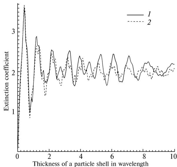
FIG. 3. Dependence of the extinction factor of the hollow particle with  $n_1 = 1$ ,  $\kappa_1 = 0$ ,  $n_2 = 1.52$ ,  $\kappa_2 = 0$  on the cover thickness 1)  $r = 5 \mu\text{m}$ ; 2)  $r = 50 \mu\text{m}$ .
