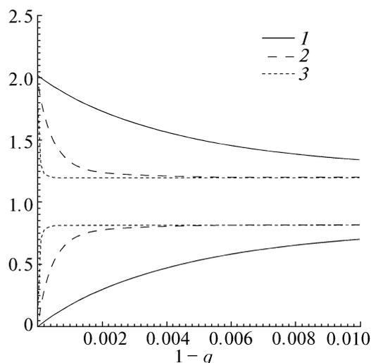
FIG. 2. Dependence of the scattering (curves above unit level) and absorption (curves below unit level) factors of particles with  $n_1 = 1.33$ ,  $\kappa_1 = 0$ ,  $n_2 = 1.74$ ,  $\kappa_2 = 0.73$  on the cover thickness 1)  $r = 25 \mu\text{m}$ ; 2)  $r = 250 \mu\text{m}$ ; 3)  $r = 2500 \mu\text{m}$ .
