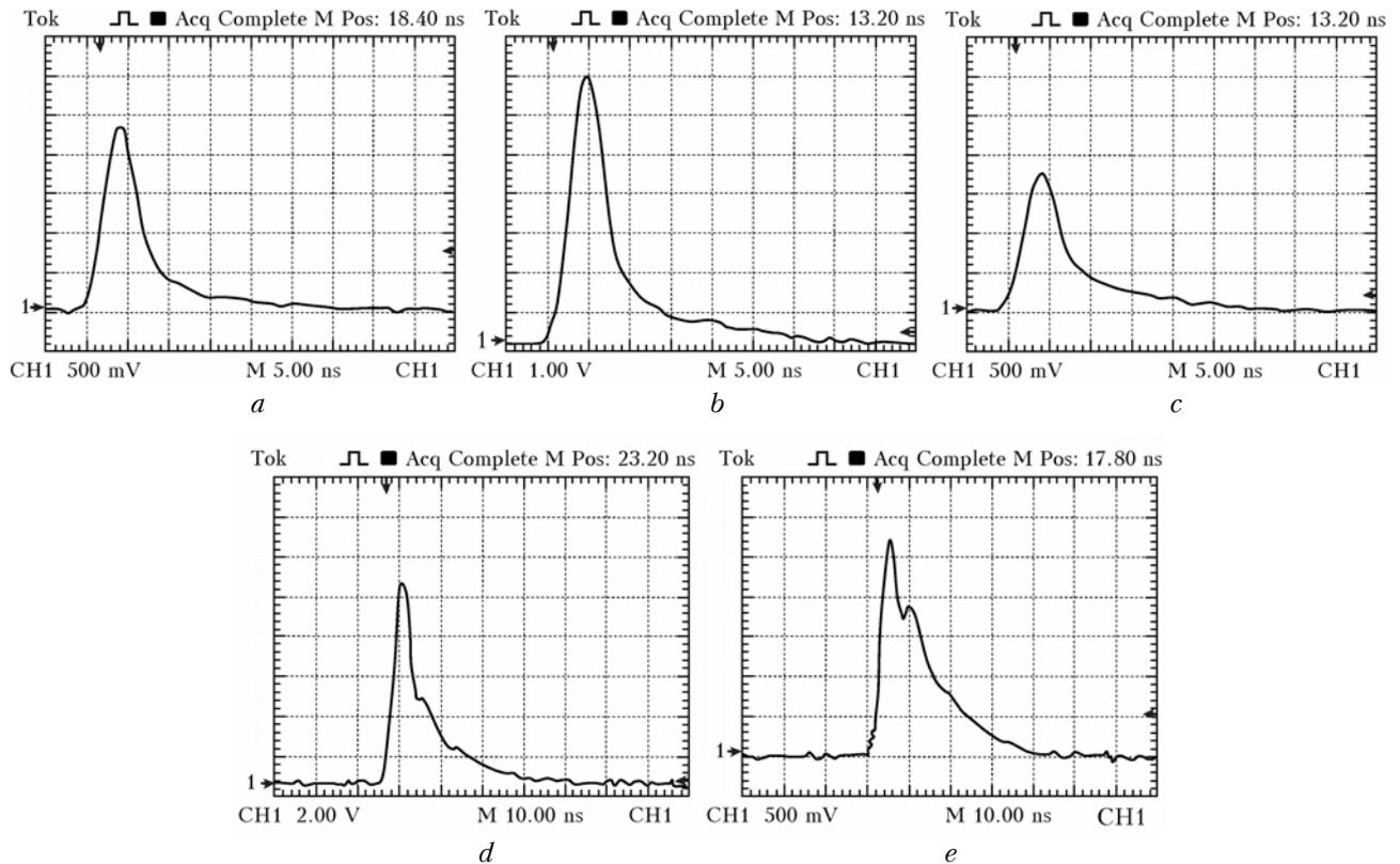
Fig. 4. The ASE pulse waveform  $r_1$  for different values of pulse compression
