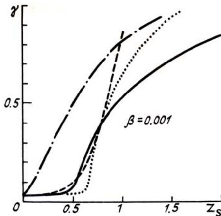
FIG. 3. The angular divergence  $\gamma$  as a function of  $z_s$  with nonlinearity of the wind type.  $f(z)$  is given by Eq. (6): collimated beam (dot-dashed curve), beam with predistortion  $\varphi_k$  (dashed curve), optimally focused beam (dotted curve);  $f(z)$  represented by Eq. (5): optimally focused beam (solid curve).
