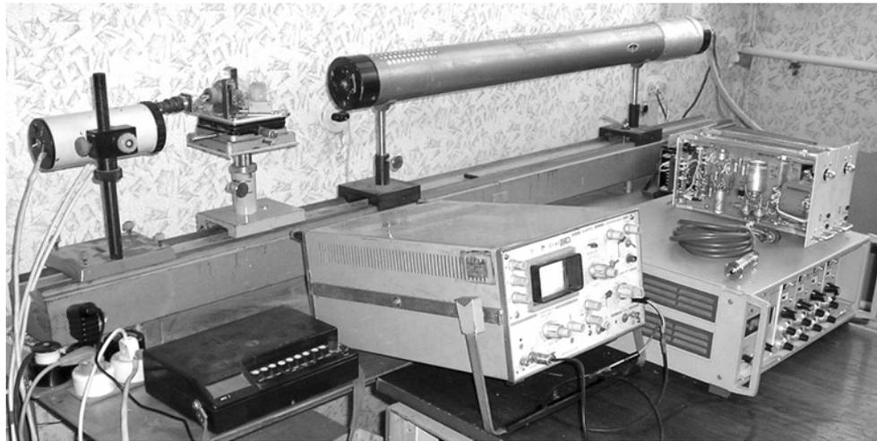
Fig. 3. External view of the three-wavelength laser with photodetection block.
