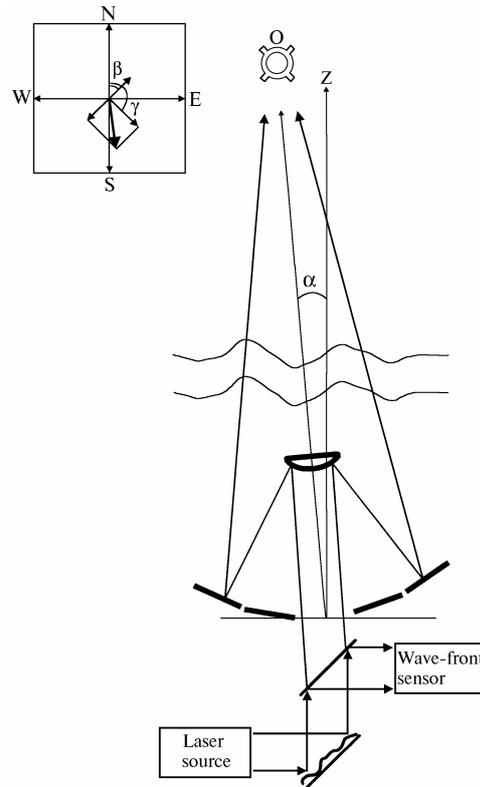
FIG. 1. Scheme of the experiment simulated numerically (construction of an image of a remote object O with the use of an adaptive telescope):  $\alpha$  is the receiver zenith angle,  $\beta$  is the scanning angle, and  $\gamma$  is the wind direction.
