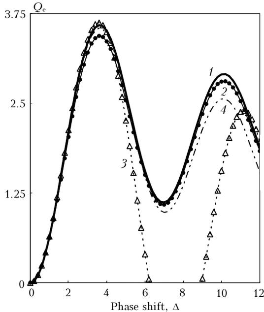
**Fig. 1.** Dependence of the extinction efficiency factor  $Q_e$  on the phase shift  $\Delta$  for infinitely long non-absorbing cylinder with relative refractive index  $m = 1.1$  (curve 1) and using the WKB scattering amplitudes in the optical theorem:  $f(\beta)$  (curve 2),  $f^{(1)}(\beta)$  (curve 3), and  $f^{(2)}(\beta)$  (curve 4).
