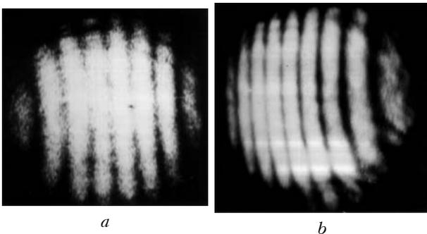
**Fig. 5.** The interference patterns recorded in the plane of hologram when it is reconstructed with a diverging spherical wave (a) and with a plane wave (b).
