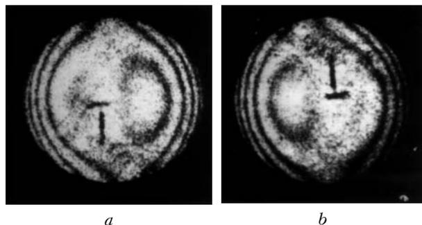
**Fig. 2.** The lateral shear interferograms characterizing the convergent wave front in the case of reconstruction of the hologram using the radiation with a diverging spherical wave (*a*) and with a plane wave (*b*).
