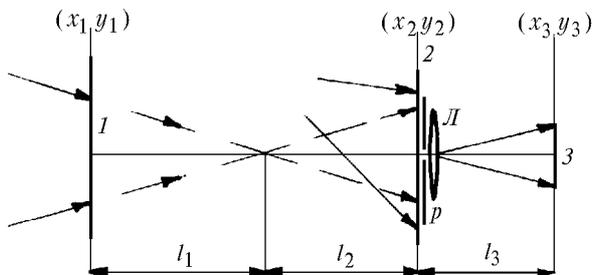
Fig. 1. The diagram of recording and reconstruction of the double-exposure hologram: mat screen (1); photoplate-hologram (2); plane of the interferogram recording (3); aperture diaphragm (p); lens (L).
