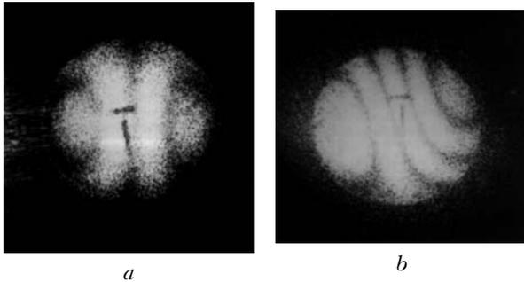
**Fig. 4.** The lateral shear interferograms characterizing the diverging wave front in the case of reconstruction of the hologram by the radiation with a diverging spherical wave (a) and with a plane wave (b).
