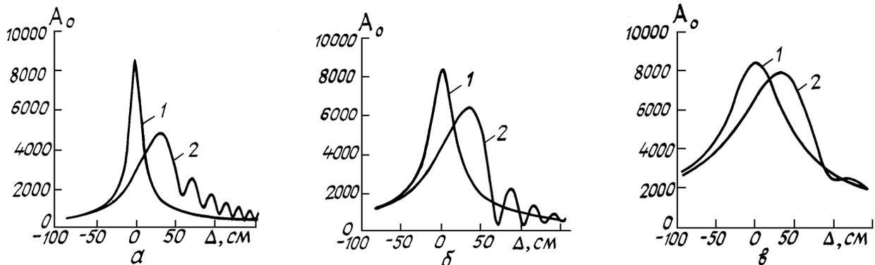
FIG. 2. Dependence of amplitude  $A_0$  on the value  $\Delta$  (1) PA and 2) exact solution) at different values of the geometrical divergence  $\alpha = a/f$ :  $\alpha = 2/30$  (a),  $2/45$  (b), and  $2$  cm/70 cm (c). The boundary beam is of Gaussian type and  $m = 1.5$ .
