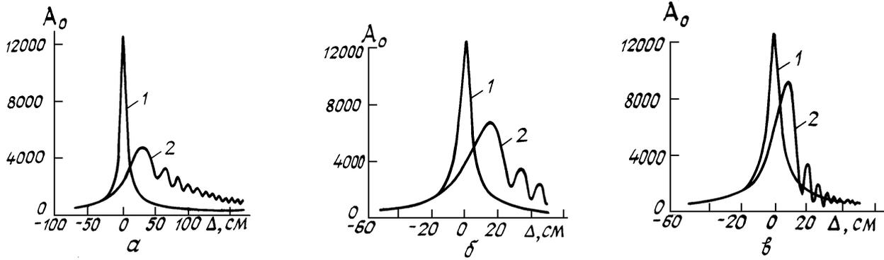
FIG. 3 Dependence of amplitude  $A_0$  on the value  $\Delta$  (1) PA and 2) exact solution) at a fixed geometrical divergence  $\alpha = (a/n)/(f/n) = 2/20$ :  $n = 1$  (a), 3 (b), and 9 (c). The boundary beam is of Gaussian type and  $m = 1.5$ .
