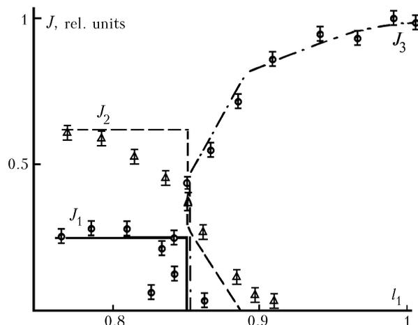
FIG. 2. Relative intensity of the components generated vs the distance between the diffraction grating and the objective.
