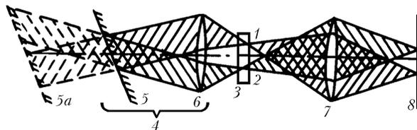
FIG. 1. Optical arrangement of the polychromatic dye laser.
