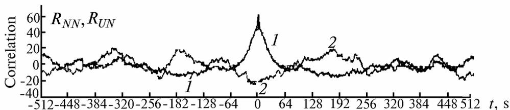
FIG. 2. Autocorrelation function of lidar signal (1) and cross-correlation function of the same signal with tangent wind velocity component (2), both normalized to the variance and multiplied by 100.
