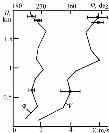
FIG. 12. The profiles of wind velocity and direction in drizzle, as measured by three–path lidar. The horizontal bars show the confidence interval at a probability of 0.95.
