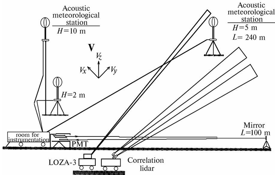
FIG. 1. Scheme of the laser-acoustic experiment to study atmospheric aerosol.
