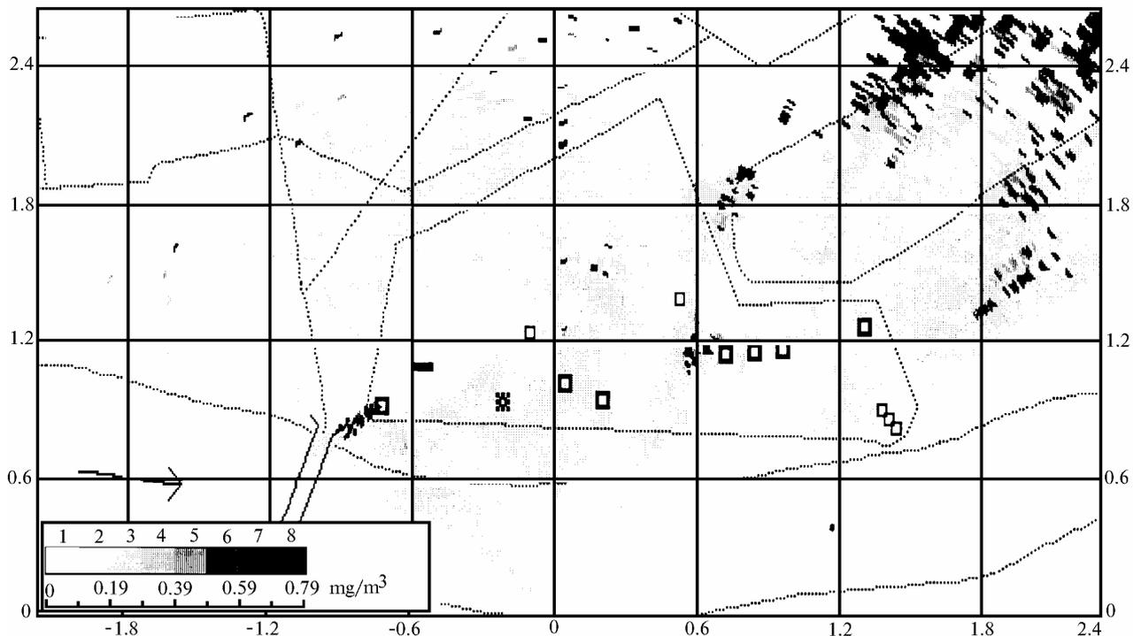
FIG. 8. Mapping of aerosol pollution distribution in azimuth scanning at angle of  $10^\circ$  at Kemerovo. The location of lidar is marked as 0 on the ordinate.
