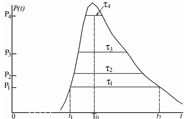
FIG. 13. The diagram of return record by a satellite laser range finder with four threshold layers.
