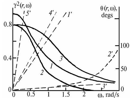
FIG. 6. The behavior of coherence and phase spectra in the presence of intense wind velocity fluctuations (theoretical calculation): coherence spectrum (1–3) and phase spectrum (1'–3'); for  $V_0 = 2$  m/s:  $\sigma_0/V_0 = 0$  (4'), 0.5 (1 and 1'), and 5 (3 and 3'); and for  $V_0 = 0.5$  m/s:  $\sigma_0/V_0 = 0$  (5') and 10 (2 and 2').
