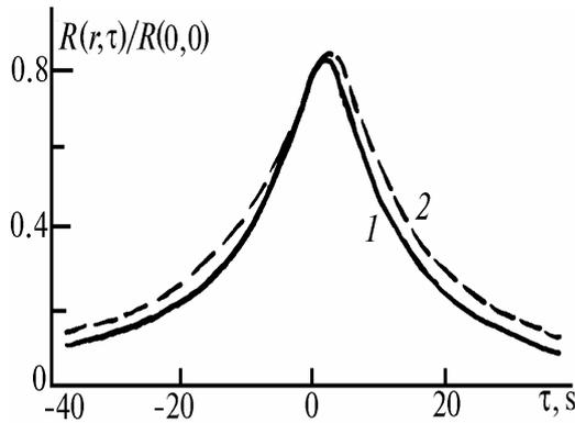
FIG. 5. The influence of anisotropy of wind velocity on cross-correlation function of lidar signal:  $\sigma_x = \sigma_y = \sigma_z = \sigma$  (1) and  $\sigma_x = \sigma_y = \sigma$ ,  $\sigma_z = 0$  (2).
