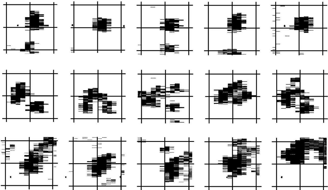
FIG. 9. Vertical sections of electric-power-station smoke plume vs. time (time interval of 2 min) and distance from stack mouth of 50 (upper row), 100 (middle row), and 150 m (lower row). The size of map grid is 75×75 m.
