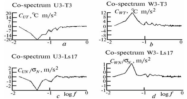
FIG. 4. Co-spectra of horizontal heat flows (a) and aerosol content (c), and the corresponding vertical flows of these quantities (b and d).
