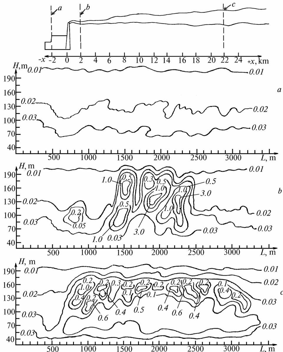
FIG. 10 The vertical distribution of mass concentration (in relative units) of aerosol near Amursk, observed on December 18, 1990: windward side (a), 2 km away from stacks (b), and 22 km away from stacks (c); uppermost section shows the scheme of experiment.
