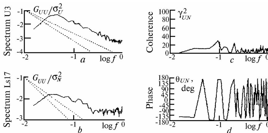
FIG. 3. Normalized autospectra of tangent wind velocity (a) and lidar signal (b), and the functions of coherence (c) and phase (d).
