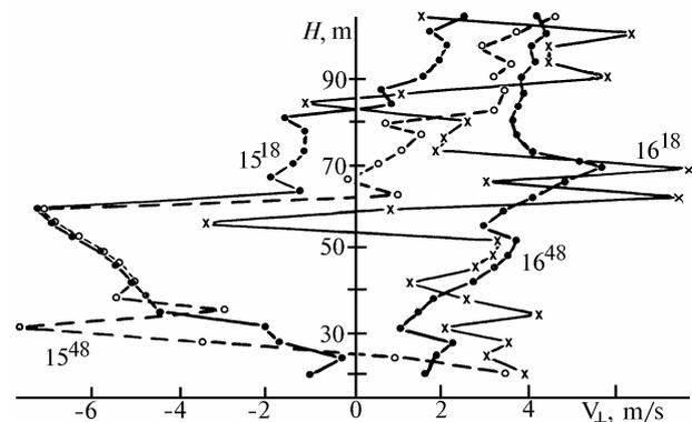
FIG. 11. Vertical wind profiles as obtained by correlation lidar when sensing along slightly inclined path over city. Numbers near curves indicate local time of measurement. Right-hand side profiles refer to wind directions from 0 to 180° and left-hand side corresponds to directions from 180 to 360°.
